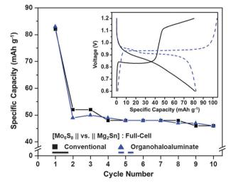
Fig. 3 The first 10 cycles for a  $[Mo_6S_8$ -conventional electrolyte- $Mg_2Sn]$  full-cell (■ black) and a [Mo<sub>6</sub>S<sub>8</sub>-organohaloaluminate electrolyte-Mg<sub>2</sub>Sn] full-cell (▲ blue); inset – 1st cycle voltage profiles for each full-cell.
