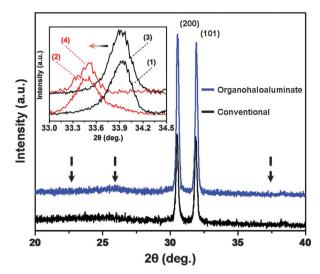
Fig. 4 XRD spectra of de-magnesiated Mg<sub>2</sub>Sn from organohaloaluminate (blue) and conventional (black) electrolytes (Mg<sub>2</sub>Sn peak positions marked with arrows). Inset - XRD spectra showing a peak shift due to magnesiation (red) of  $Mo_6S_8$  (black) in organohaloaluminate (peak shift 1  $\rightarrow$  2) and conventional (peak shift  $3 \rightarrow 4$ ) electrolytes.
