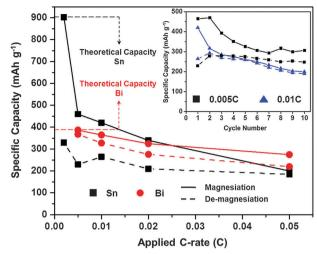
Fig. 2 Magnesiation/de-magnesiation capacities for Sn/Mg (■ black) and Bi/Mg ( red) half-cells at various C-rates. All half-cells were tested using an organohaloaluminate electrolyte. Inset – 10 cycles of a Sn/Mg half-cell at 0.005 C (■ black) and 0.01 C ( blue) rates in the same electrolyte.
