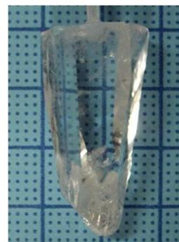
Fig. 1 GAB crystal grown by TSSG method in  $\text{Al}_2\text{O}_3\text{--B}_2\text{O}_3\text{--Li}_2\text{O--NaF}$  flux
