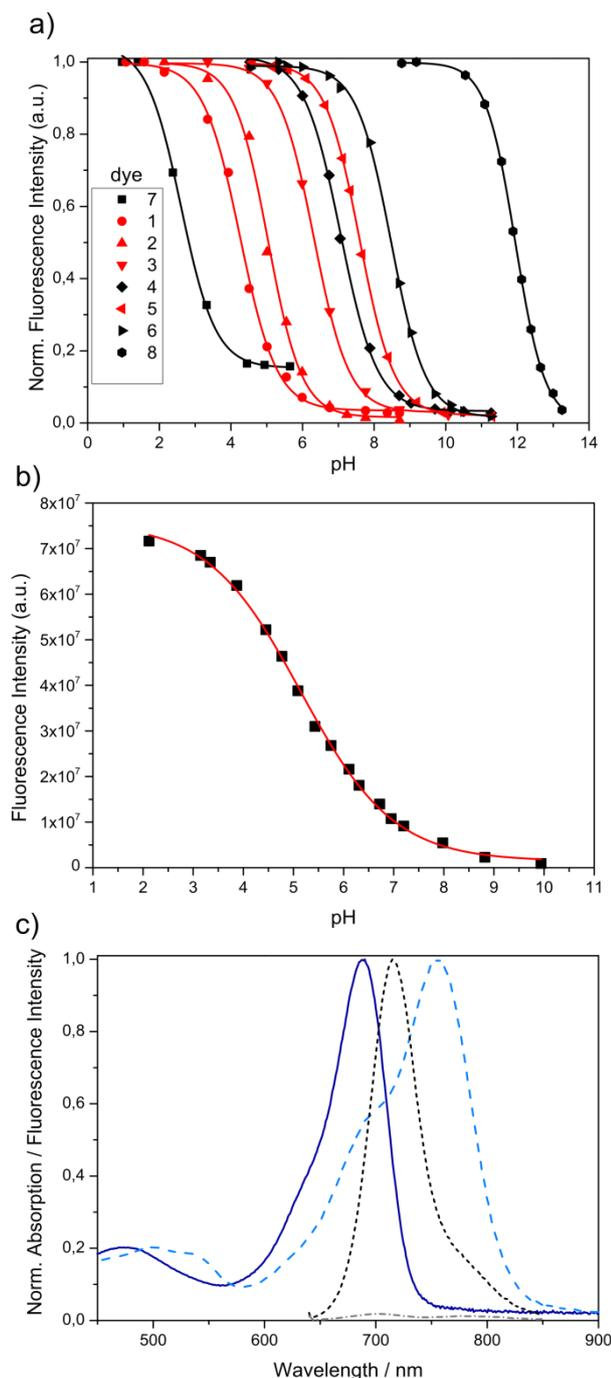
Figure 1 a) Calibration curves of probe 1-8, determined in D4 from emission spectra. Combination of probe (1,2,3,5) (red) in D4 yields a broad-range sensor (b) with an extended dynamic range from pH 2 to 9. c) Absorption of protonated (blue) and deprotonated (dashed-blue) form and fluorescence (dotted black) of the broad-range sensor.
