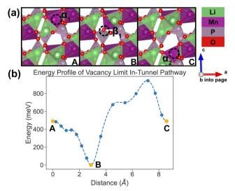
Fig. 8 Li vacancy evolution of the along-tunnel pathway (Pathwayl) in the vacancy limit. (a) Shows images along the pathway, where dashed circles indicate positions of vacancies; vacancy positions labeled  $\alpha_1$ ,  $\beta_1$  and  $\alpha_2$ have the same positions with identical labels in Fig. 4. (b) Shows calculated energy evolution as a function of vacancy migration distance, where labels  $\alpha_1$ ,  $\beta_1$  and  $\alpha_2$  correspond to the images in (a).
