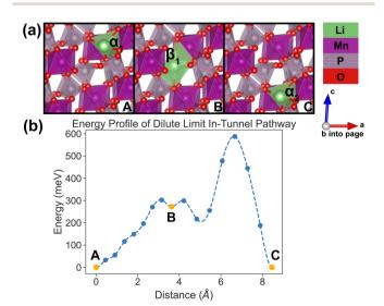
Fig. 6 Li-ion evolution of the along-tunnel pathway (Pathwayl) in the dilute limit. (a) Shows images along the pathway, and Li positions labeled  $\alpha_1$ ,  $\beta_1$  and  $\alpha_2$  have the same positions with identical labels in Fig. 4. (b) Shows calculated energy evolution as a function of Li migration distance, where labels  $\alpha_1$ ,  $\beta_1$  and  $\alpha_2$  correspond to the images in (a).
