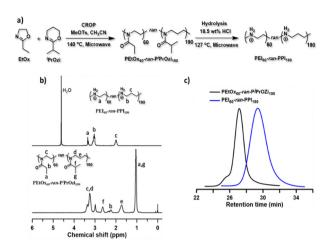
Fig. 1 Overview copolymer synthesis and analysis. Panel (a): synthesis scheme for the preparation of L-PEI<sub>60</sub>-ran-PPI<sub>190</sub> copolymer. Panel (b):  $^{1}$ H NMR spectra of PEtOx $_{60}$ -ran- $\mathrm{P^{i}PrOzi}_{190}$  and L-PEI $_{60}$ -ran-PPI $_{190}$  in CDCl<sub>3</sub> and D<sub>2</sub>O, respectively. Panel (c): SEC traces of PEtOx<sub>60</sub>-ran-PiPrOzi<sub>190</sub> in DMA and L-PEI<sub>60</sub>-ran-PPI<sub>190</sub> in aqueous medium.
