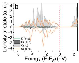
Fig. 1 The partial density of states of the valence bands of (a)  $CrSe_2$  and (b)  $KCrSe_2$ . The Fermi energy  $E_F$  is given by a dashed line.
