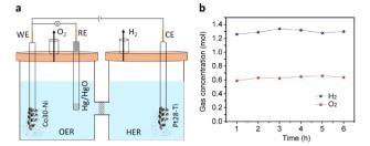
Fig. 4 (a) Schematic diagram illustrating a full-cell alkaline water electrolyser with swarf electrodes Pt28-Ti and Co30-Ni operating as electrocatalysts for the HER and OER, respectively. (b) Evolution of oxygen and hydrogen from the cell over time.
