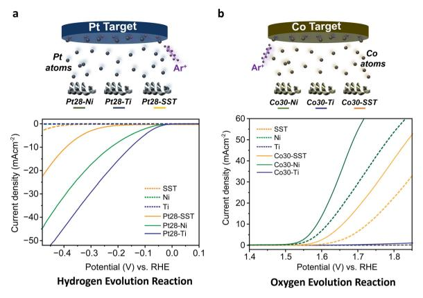
**Xp-Y** where **X** type of metal catalyst and **p** the amount of **X** in μg cm<sup>-2</sup>, and **Y** is the type of swarf.
