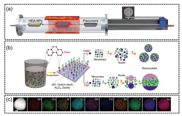
Fig. 6 FMBP synthesis from the work of Gao et al., (a) illustration of the FMBP experimental setup to synthesize HEA NPs from precursors, (b) schematics for the synthesis of HEA NPs which are homogeneous when synthesized via FMBP, and phase-separated when synthesized via fixed bed pyrolysis (FBP), and (c) STEM-EDX elemental mapping of MnCoNiCuRhPdSnIrPtAu constituents. The scale bar is 10 nm. Reproduced with permission.105 Copyright Springer Nature 2020
