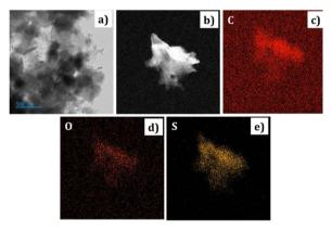
**Fig. 4** (a) HR-TEM image of PEDOT (b) secondary electron image in EDS elemental mapping of PEDOT (c) carbon in PEDOT (d) oxygen in PEDOT (e) sulphur in PEDOT.
