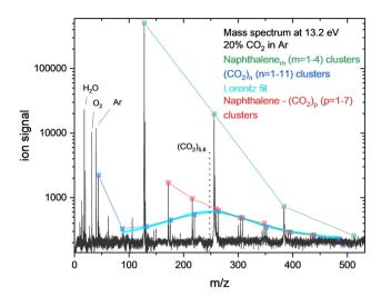
Fig. 4 Mass spectra at 13.2 eV photon energy (black) where least fragmentation of pure  $CO_2$  clusters is expected (see Fig. 3). Indicated are the pure  $CO_2$  clusters (dark blue), the naphthalene clusters (green) and the naphthalene– $CO_2$  clusters (red). A Lorentz fit of the pure  $CO_2$  cluster size distribution (light blue), not including the monomer, indicates a mean cluster size of 5.6  $CO_2$  units.
