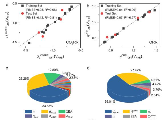
Fig. 6 Comparison between DFT-calculated and ML-predicted values of (a)  $U_{\rm L}^{\rm CO_2RR}$  and (b)  $\eta^{\rm ORR}$ . Feature importance for (c)  $U_{\rm L}^{\rm CO_2RR}$  in the GBR model and (d)  $\eta^{\text{ORR}}$  in the XGBoost model.
