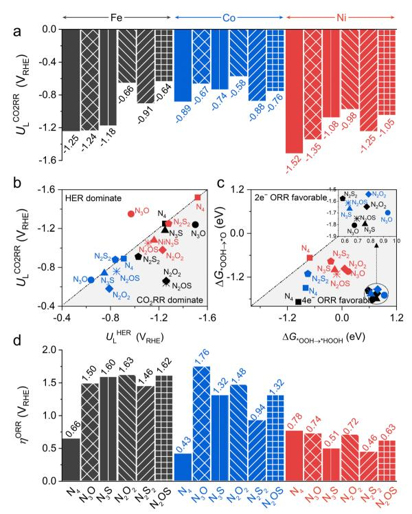
Fig. 4 (a) Limiting potential of  $CO_2RR$ -to-CO of  $Fe/Co/Ni-N_xO_yS_z$ -Por-COFs. (b) Limiting potential of  $CO_2RR$ -to-CO vs. limiting potential of HER. (c) Gibbs free energy changes (∆G\*OOH → \*O) of \*O formation vs. Gibbs free energy changes (∆G\*OOH → HOOH) of HOOH formation. (d) Overpotential of ORR-to- $H_2O$  of Fe/Co/Ni- $N_xO_vS_z$ -Por-COFs.
