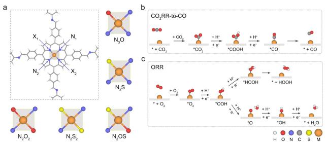
Fig. 1 (a) Unit cell of the  $M-N_4$ -Por-COF (M = Fe/Co/Ni) considered in this work and the constructed  $N_xO_yS_z$  coordination models. Reaction pathways for (b)  $CO_2RR$ -to-CO and (c) ORR-to- $H_2O_2$  ( $2e^-$ )/ $H_2O$  ( $4e^-$ ).
