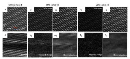
Fig. 8 The schematic illustration of CS and the reconstructed images. Images of NiTiO<sub>3</sub> acquired under (a) fully, (b) 50%, and (c) 20% sampled conditions. Reproduced with permission.<sup>78</sup> Copyright 2016, AIP Publishing. Images of the complex perovskite sample acquired under (d) fully, (e) 50%, and (f) 20% sampled conditions. Reproduced with permission.<sup>79</sup> Copyright 2016, AIP Publishing
