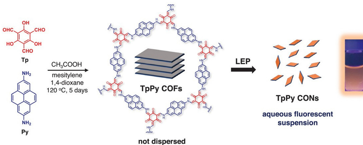
Fig. 2 Schematic diagram of the preparation of TpPy CONs by solvothermal condensation and liquid exfoliation process (fluorescent photograph of a 0.5\text{ mg mL}^{-1} TpPy CON dispersion taken under 365\text{ nm} UV light). Adapted with permission from ref.79.
