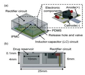
**Fig. 9** IPMC-based cantilever valve for drug delivery. The body of the device is made of biocompatible polydimethylsiloxane (PDMS) and has external dimensions of 15 mm  $\times$  25 mm  $\times$  6 mm, including drug storage with a maximum loading capacity of 520  $\mu$ L. (a) Schematic illustration of the drug delivery device; (b) side view of the drug delivery device. Reproduced with permission. <sup>95</sup> Copyright 2018 Royal Society of Chemistry.
