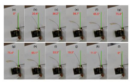
Fig. 1 (a)-(f) Bending response images of an IPMC actuator under the same DC voltage; (g)-(l) recovery process diagram after removing the voltage.
