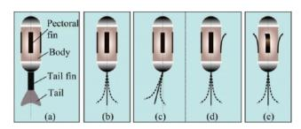
Fig. 10 The mechanical structure of a capsule-like robot and motion control principle. (a) Mechanical structure; (b) swim forward; (c) turning by asymmetric swing of caudal fin; (d) turning by opening of pectoral fin; (e) positioning. Reproduced with permission. 105 Copyright 2020 Springer.
