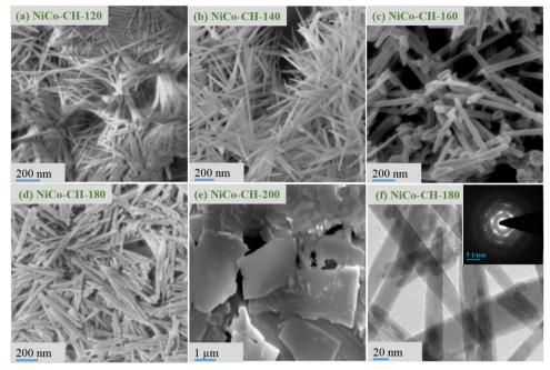
Fig. 2 FESEM images of NiCo-CH synthesized at a solvothermal temperature of (a)  $120 \,^{\circ}$ C, (b)  $140 \,^{\circ}$ C, (c)  $160 \,^{\circ}$ C, (d)  $180 \,^{\circ}$ C, and (e)  $200 \,^{\circ}$ C while other parameters are fixed (2:1 Ni: Co precursor, 15 mL EG + 20 mL water, 12 h). (f) TEM image of the sample NiCo-CH-180 obtained at 180  $\,^{\circ}$ C and the inset shows the SAED pattern of the corresponding sample.
