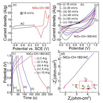
Fig. 6 (a) CV curve of the negative (AC) and positive (NiCo-CH-180) electrode at 10 mV s<sup>-1</sup> in a three-electrode set up. (b) CV curves for the ASC at various scan rates (10-100 mV s), (c) GCD curves at different current densities (2-10 A g<sup>-1</sup>), and (d) Nyquist plot of the NiCo-CH-180// AC ASC (two-electrode device)
