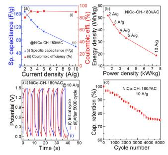
Fig. 7 (a) Specific capacitance and coulombic efficiency of NiCo-CH-180//AC ASC at different current densities (2-10 A g<sup>-1</sup>), (b) Ragone plot (ED vs. PD), (c) initial and after 5000 charge-discharge curves, and (d) capacitance retention performance up to 5000 charge-discharge cycles at 10 A  $\rm g^{-1}$  current density of the NiCo-CH-180//AC ASC.
