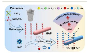
Fig. 1 Schematic illustration of the fabrication of HAP@FAP.
