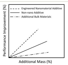
Fig. 1 Material efficiency is the concept in which the ratio of functional gain to material mass increases compared with a baseline, alternative, or status quo. This figure illustrates the concept for engineered nanomaterials wherein the gain in function of the bulk material per unit nanomaterial mass added is much larger than for non-nanomaterial approaches. The slope indicates the material efficiency and the linear trends are demonstrative.
