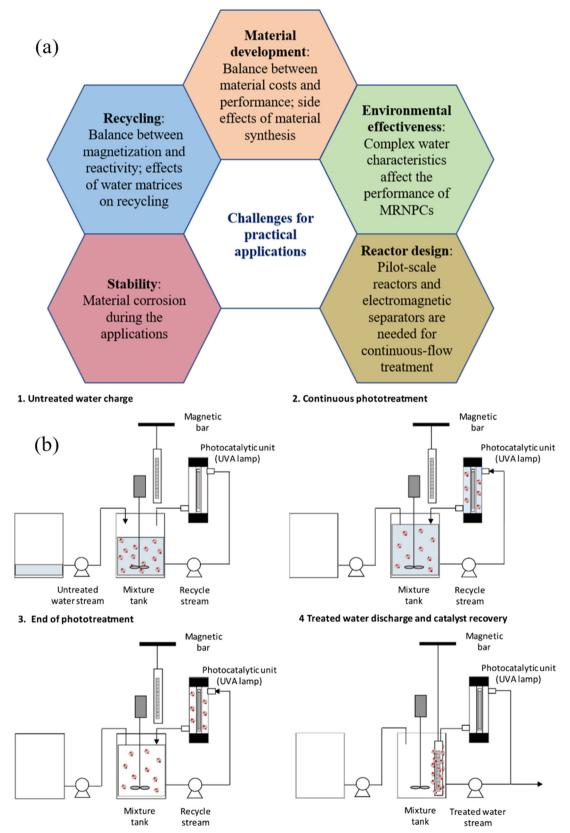
Fig. 8 (a) Challenges of MNRPCs in practical applications; (b) operation of magnetic photocatalytic reactor: 1) loading of MNRPCs and water, 2) continuous phototreatment; 3) end of phototreatment, 4) MNRPCs recycling. Reproduced from ref. 70 with permission from Elsevier, copyright 2019.
