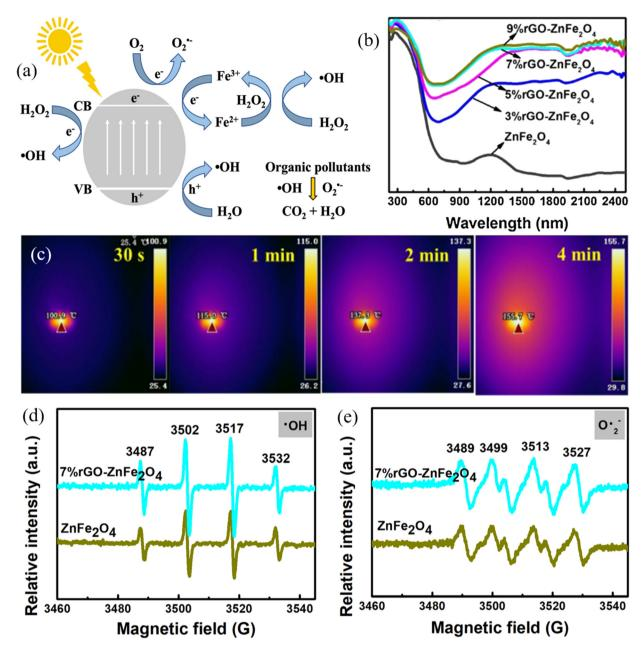
Fig. 5 (a) Schematic diagram showing the mechanism of photocatalytic-Fenton like process using MRNPCs; (b) light adsorption spectra of different rGO- $ZnFe_2O_4$  samples; (c) infrared thermal image of 7% rGO- $ZnFe_2O_4$  under solar light illumination; generation of (d) 'OH and (e)  $O_2$ ' by  $ZnFe_2O_4$  and 7% rGO- $ZnFe_2O_4$  in the photocatalytic-Fenton like processes. Reproduced from ref. 131 with permission from Elsevier, copyright 2021.
