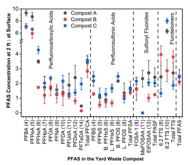
Fig. 3 The ratio of PFAS concentrations at 2 ft depths to the surface in the yard waste compost. To calculate the ratio, PFAS concentrations at 2 ft depths were divided by the PFAS concentrations at the surface for composts A, B, and C. Nineteen out of the forty analyzed PFAS were detected in these compost samples.
