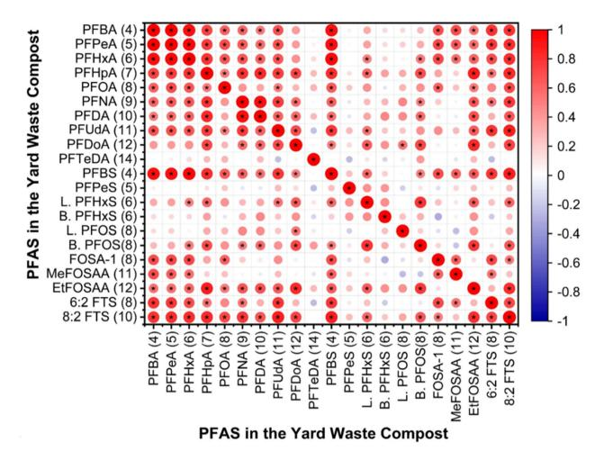
Fig. 5 Pearson correlation (significant at  $\alpha \le 0.05$ ) among the detected PFAS at the surface level (i.e., 0 ft) and at 2 ft depths in yard waste composts A, B, and C. The red circle with '\*' denotes a significant correlation between the corresponding pairs of the PFAS. The red color in the right-side bar indicates the intensity of a strong correlation, and the blue color denotes the intensity of a weak correlation among different PFAS.
