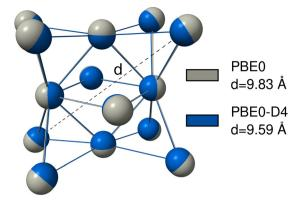
Fig. 8 PBE0/def2-SVP (grey) and PBE0-D4/def2-SVP (blue) optimized No<sub>14</sub>-cluster. PBEO-NL/def2-SVP is hidden for better visibility, however, the result is very similar to the D4 result with d = 9.55 Å. The calculated diagonal distance is shown as the dashed black line.
