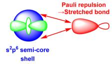
Fig. 10 Schematic representation of the origins of the 'Pauli shield'. (After Fig. 3 of ref. 41.) The (n-1)s, (n-1)p and (n-1)d orbitals on the metal have comparable radii and the red double-headed arrows indicate the Pauli repulsion from the electrons in the filled s and p semi-core orbitals on the electron pair in the ligand  $\sigma$  bond (red).
