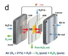
Fig. 5 Different types of setups for H<sub>2</sub>O<sub>2</sub> production. (a) One-pot setup. Reproduced from ref. 11. Copyright (2022) Elsevier. (b) H-cell. (c) Illustration of the flow cell setup. Reproduced from ref. 17. Copyright (2021) Wiley-VCH GmbH. (d) solid-electrolyte (SE) cell system. Reproduced from ref. 78. Copyright (2023) Wiley-VCH GmbH.
