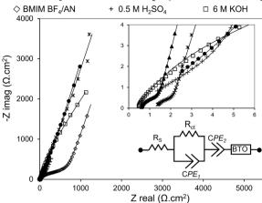
Fig. 8 EIS measurements of coal char electrodes presented as a normalized Nyquist plot. Upper inset: High-frequency behavior. Lower inset: Randles equivalent circuit model with series resistance  $R_{s_r}$  charge transfer resistance  $R_{ct}$ , constant phase elements (CPE<sub>1</sub> and CPE<sub>2</sub>), and Bisquert Open (BTO) circuit elements
