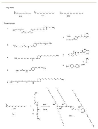
Fig. 15 Structures of the alkyl chains (A) and polyamine cores (B) were used to generate the ionizable lipid library. (C) C14-4 is used here as a representative reaction.
