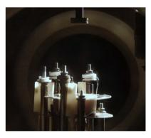
Fig. 1 Close-up visualization of the i-PLD heating stage as well as a photograph inside of the PLD chamber with a mounted target.
