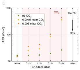
Fig. 7 Effect of *in situ* decoration from a Sr-containing target on the area specific surface exchange resistance of a dense LSC thin film at (a) high (600 °C) and (b) low (450 °C) temperatures in 0.04 mbar  $O_2$  for different amounts of additional  $CO_2$  introduced into the chamber. The arrow indicates a slow but continuous recovery of the area specific surface exchange resistance after  $CO_2$  was turned off.
