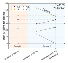
Fig. 5 Surface chemistry of LSC decorated with 1 monolayer of SrO at high temperature compared with LSC decorated with 1 monolayer SrO at low temperature before and after heating to 600 °C inside the XPS chamber. All measurements were performed at 450 °C and 7  $\times$  10<sup>-6</sup> mbar oxygen.
