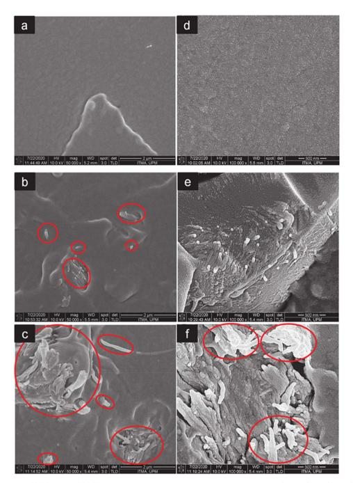
Fig. 12 FESEM images at  $500\,00\times$  and  $1\,000\,00\times$  magnification of the fractured surfaces of neat PLA (a and d), PLA/CNF3 (b and e), and PLA/CNF6 (c and f), respectively. Red circles show nanocellulose. PLA/CNF6 exhibits agglomerated nanocellulose. CNF: nanocellulose. Number after CNF indicates the % against the weight of PLA.<sup>60</sup>
