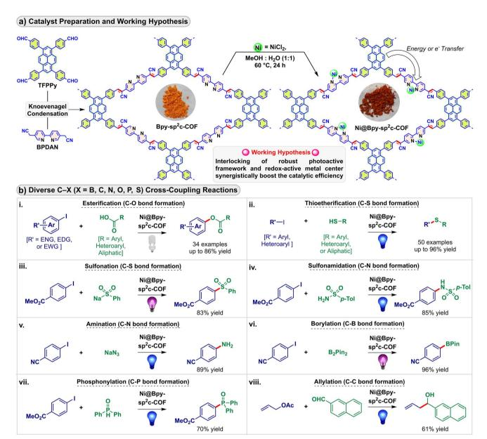
Fig. 1 (a) Catalyst preparation via NiCl<sub>2</sub> installation in the Bpy-sp<sup>2</sup>c-COF and the working hypothesis; and (b) application of the Ni@Bpy-sp<sup>2</sup>c-COF catalyst in different C-X (X = B, C, N, O, P, S) cross-coupling reactions with isolated yields of the products. ENG = electron neutral group, EDG = electron donating group, EWG = electron withdrawing group.
