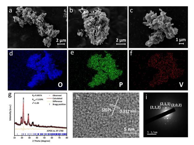
Fig. 1 (a-c) SEM images, (d-f) elemental mappings, (g) Rietveld XRD pattern, (h) HR-TEM and (i) SAED images of δ-VOPO<sub>4</sub>.
