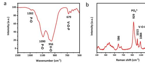
Fig. 2 (a) FTIR spectra and (b) Raman spectra of  $\delta$ -VOPO<sub>4</sub> powder.
