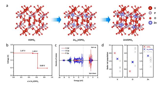
Fig. 5 (a) The schematic illustration of structural models of  $\delta$ -VOPO<sub>4</sub> before and after dezincification; (b) the equilibrium reaction voltage profiles predicted with DFT calculations; (c) the density of states (DOS) of  $\delta$ -VOPO<sub>4</sub>; the Fermi energy level is set to zero; (d) the Bader charge analysis of  $\delta$ -VOPO<sub>4</sub>.
