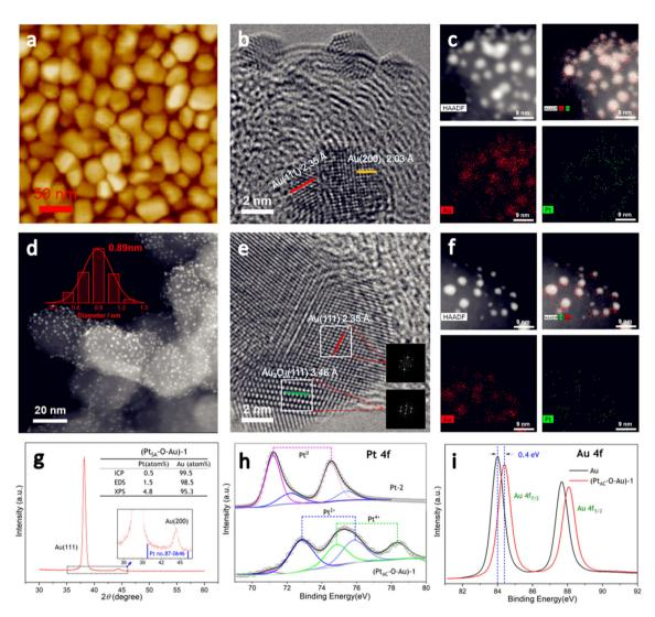
Fig. 1 The AFM, HRTEM, HAADF-STEM images and STEM-EDS elemental maps of the  $(Pt_{AC}-Au)$ -1 electrode (a-c). The HAADF-STEM images of the Pt-1 electrode (d). The HRTEM, HAADF-STEM images and STEM-EDS elemental maps of the  $(Pt_{AC}-O-Au)$ -1 electrode (e-c) and (e-c) and
