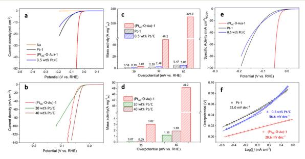
Fig. 2 The apparent HER activities of (Pt<sub>AC</sub>-O-Au)-1, Pt-1, 0.5 wt% Pt/C and Au (a). The apparent HER activities of (Pt<sub>AC</sub>-O-Au)-1, 20 wt% Pt/C and Au (a). 40 wt% Pt/C (b). The MAs of (Pt<sub>AC</sub>-O-Au)-1, Pt-1, 0.5 wt% Pt/C, 20 wt% Pt/C and 40 wt% Pt/C (c and d). The SAs of (Pt<sub>AC</sub>-O-Au)-1, Pt-1 and 0.5 wt% Pt/C (e). The Tafel slopes of (Pt<sub>AC</sub>-O-Au)-1, Pt-1 and 0.5 wt% Pt/C (f).
