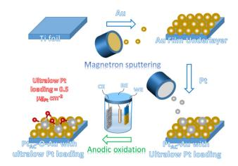
Scheme 1 Schematic illustration of the preparation of Pt<sub>AC</sub>-O-Au.
