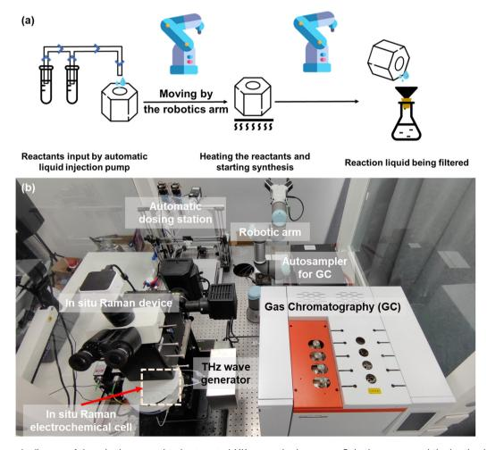
Fig. 2 (a) Schematic diagram of the robotic-arm-assisted automated MXene synthesis process. Robotic arms moved the heating kettle for safety due to the HF generated during the process. (b) Physical map of the robotic-arm-assisted electrolyte preparation device, electrocatalytic reaction device (in situ Raman electrochemical cell), and in situ Raman and GC test setup. The THz wave generator was a model CQ-8 THz electromagnetic wave therapy device.27
