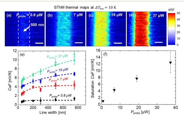
Fig. 3 (a–d) SThM thermal maps of a 500 nm wide metal line at  $\Delta T_{\rm line} = 10$  K when scanning at probe powers ( $P_{\rm probe}$ ) of (a) 0.8  $\mu$ W, (b) 7  $\mu$ W, (c) 19  $\mu$ W, (d) 37  $\mu$ W (scale bar equal to 400 nm). (e) Calculated calibration factor (CaF) for different power values as a function of the line width of the scanned metal lines (upwards triangle correspond to the retrace signal). (f) Estimated saturated CaF as a function of  $P_{\rm probe}$ .
