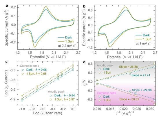
Fig. 3 Electrochemical performance of Cu-HHB electrodes both in the dark and 1 sun illuminated conditions. (a and b) CV profiles at 0.2 mV s<sup>-1</sup> and 1 mV s<sup>-1</sup> in the dark and 1 sun illumination. (c) Plots of log  $(i_0)$  vs. log (v): estimation of b-values for cathodic and anodic peaks in the dark and 1 sun illumination. (d) Estimation of Li-ion diffusion constant improvements under illumination from  $I_p/N$  vs.  $v^{1/2}$  curves.
