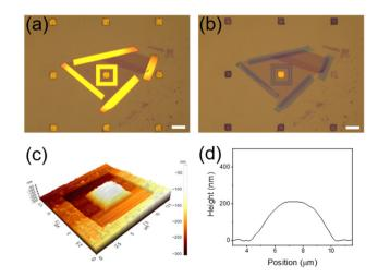
Fig. 4 Optical micrographs of Au NPCs patterns (a) before and (b) after the KCN treatment. Scale bars indicate 10 µm. (c) Atomic force microscopy image and (d) corresponding height profile of the device left under the reaction conditions for 3 h.
