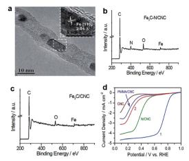
Fig. 4 (a) High resolution transmission electron microscopy (HRTEM) image of Pod-Fe with the inset showing the [110] crystal plane of Fe.  $^{25}$  XPS spectra of (b) Fe<sub>3</sub>C-N/CNC and (c) Fe<sub>3</sub>C/CNC.  $^{29}$  (d) ORR performance of Fe<sub>3</sub>C-N/CNC (curve 1) and Fe<sub>3</sub>C/CNC (curve 2).  $^{29}$
