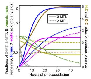
Fig. 3 Temporal evolution of aqueous atmospheric chemistry of the 2-MTS (solid lines) and 2-MT (dashed lines) systems in the optimized mechanism (Mechanism S1†) as implemented in GEOS-Chem for  ${\rm [OH]}_{\rm q}=10^6$  molecule per cm³.
