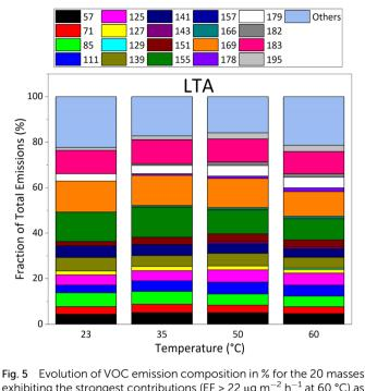
exhibiting the strongest contributions (EF > 22  $\mu$ g m<sup>-2</sup> h<sup>-1</sup> at 60 °C) as a function of temperature, as measured by PTR-ToFMS under dry (RH = 0.1%) and dark conditions, for the LTA2 old asphalt sample.
