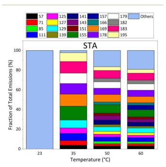
Fig. 4 Evolution of VOC emission composition in % for the 20 masses exhibiting the strongest contributions (EF > 22  $\mu$ g m<sup>-2</sup> h<sup>-1</sup> at 60 °C) as a function of temperature, as measured by PTR-ToFMS under dry (RH = 0.1%) and dark conditions, for the STA3 fresh asphalt sample.
