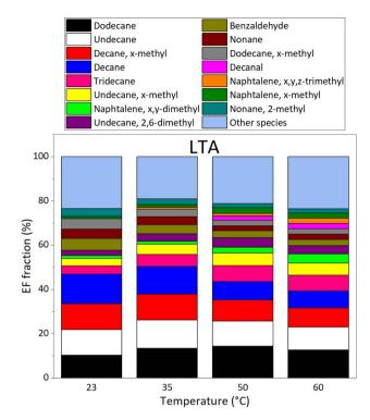
Fig. 7 Evolution of VOC emission composition in % for the species accounting for more than 75% of VOC emissions (EF > 3.63  $\mu$ g m<sup>-2</sup> h<sup>-1</sup> for LTA asphalt mixtures) as a function of temperature, as measured by GC-MS/FID under dry (RH = 0.1%) and dark conditions, for the LTA2 old asphalt sample.
