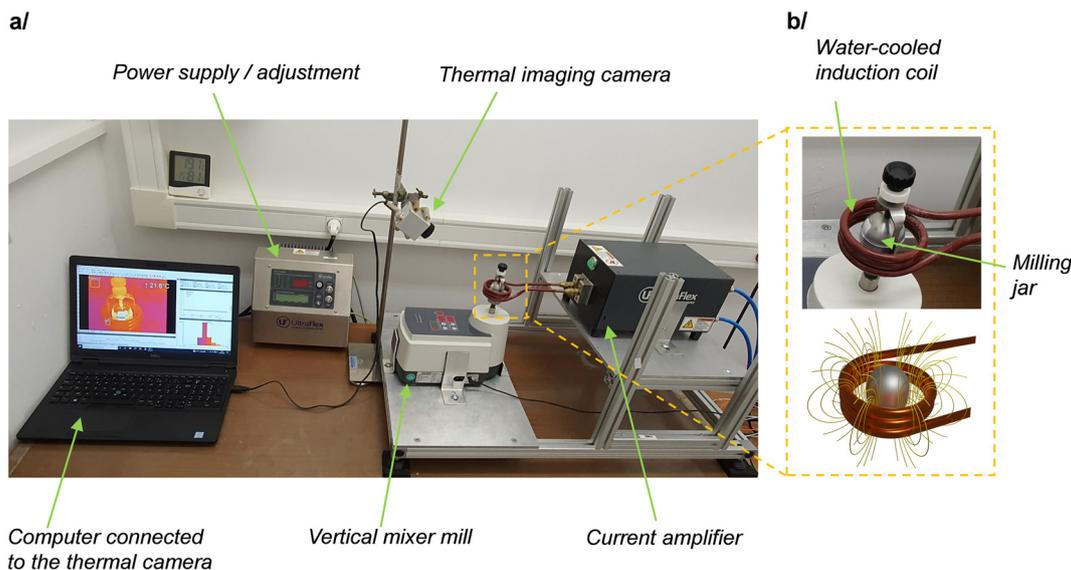
Fig. 1 (a) Representation of the experimental set-up used for induction heating during ball-milling (i-BM). (b) Zoom onto the milling jar and induction coil (top), and schematic representation of the magnetic field lines when current is circulating in the coil (bottom). Additional pictures and views of the instrumental set-up are provided in ESI† (Fig. S1).
