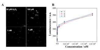
Fig. 5 (A) ECL image of  $Co_3O_4$  at ITO slides with different concentrations of  $H_2O_2$ ; the exposure time was 500 ms, and the applied potential was 1 V. (B) Correlation between the luminescence of three particles and the concentration of  $H_2O_2$ . Scale bar: 5  $\mu$ m.
