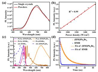
Fig. 3 (a) PL spectra of (HM)Pb $_2$ Br $_6$  crystals and powder. (b) Integrated emission intensity versus excitation power for (HM)Pb2Br6. (c) Normalized absorption, PLE and PL spectra of HMBr2 and (HM)Pb2Br6. (d) Timeresolved PL lifetime of (HM)Pb2Br6 and HMBr2 under 375 nm excitation at 298 K.
