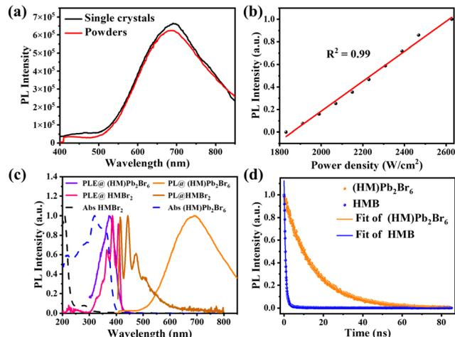
Fig. 3 (a) PL spectra of (HM)Pb<sub>2</sub>Br<sub>6</sub> crystals and powder. (b) Integrated emission intensity versus excitation power for (HM)Pb<sub>2</sub>Br<sub>6</sub>. (c) Normalized absorption, PLE and PL spectra of HMBR<sub>2</sub> and (HM)Pb<sub>2</sub>Br<sub>6</sub>. (d) Time-resolved PL lifetime of (HM)Pb<sub>2</sub>Br<sub>6</sub> and HMBR<sub>2</sub> under 375 nm excitation at 298 K.
