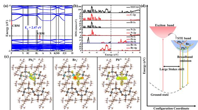
Fig. 4 (a) Calculated electronic band structures and (b) DOS of (HM)Pb<sub>2</sub>Br<sub>6</sub>. (c) Calculated charge density for (HM)Pb<sub>2</sub>Br<sub>6</sub> (Pb<sub>2</sub><sup>3+</sup>, Br<sub>2</sub><sup>-</sup> and Pb<sub>3</sub><sup>+</sup> STEs) holes upon crystal lattice perturbation via the Pb-Pb, Br-Br and Pb-Br distances shortening. (d) Configuration coordinate diagram illustrating the luminescence mechanism.
