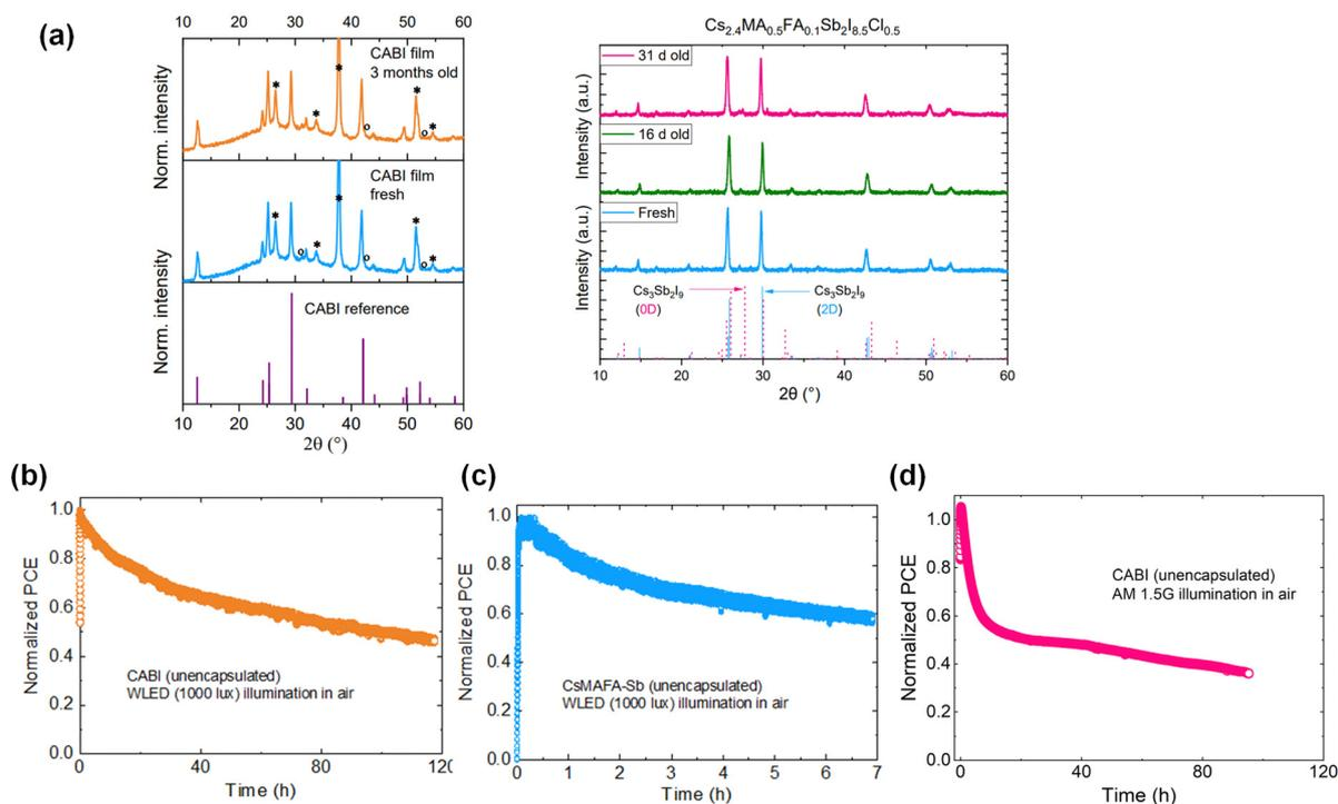
Fig. 4 (a) XRD patterns of fresh and aged CABI films stored in air (reproduced from<sup>24</sup>) and fresh and aged CsMAFA-Sb films stored in dry air (RH of 15%) (reproduced from<sup>31</sup>). MPP tracking of unencapsulated devices (in their n-i-p planar device architecture) of (b) CABI and (c) CsMAFA-Sb under WLED (1000 lux) illumination, and (d) CABI under 1-Sun illumination in air (RH ~50%).
