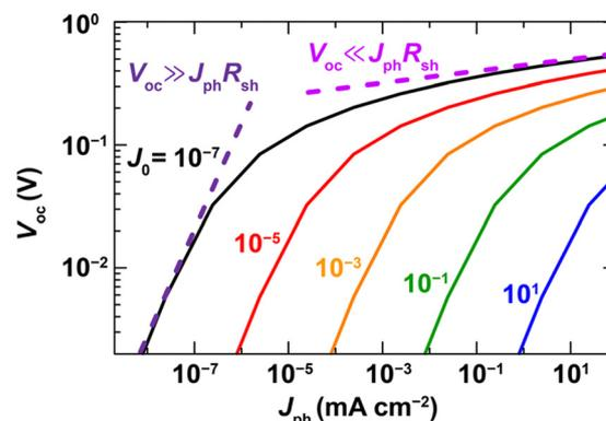
Fig. 3 The simulated graph showing how reducing the leakage current can sustain high photovoltage even under low intensity illumination (adapted from<sup>105</sup>).
