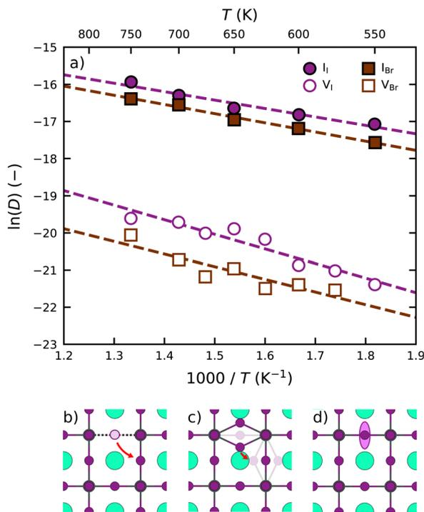
**Fig. 3** (a) Temperature evolution of self-diffusion coefficients of halide vacancies ( $V_X$ ; white symbols) and halide interstitials ( $I_X$ ; coloured symbols) in  $\text{CsPbX}_3$ . The defect migration pathways of (b)  $V_I$  and (c)  $I_I$  defects in  $\text{CsPbI}_3$ , with both the initial and final structures. (d) The typical motion of halide species in the perovskite lattice.
