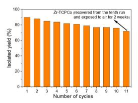
Fig. 2 Recyclability of the photocatalyst Zr-TCPCo.
