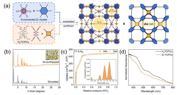
Fig. 1 (a) Schematic illustration of the design and synthesis of Zr-TCPCo with an she net; (b) PXRD patterns of Zr-TCPCo; inset: Optical micrograph of Zr-TCPCo; (c) 77 K N2 adsorption test of Zr-TCPCo; inset: diagram of incremental pore volume vs. pore width; (d) UV-vis spectra of Zr-TCPCo and the molecular cobaloxime H<sub>4</sub>TCPCo.
