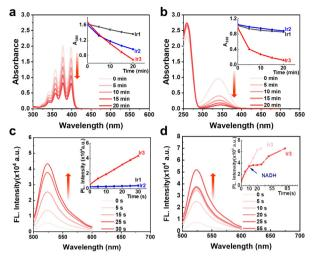
Fig. 2 Photoactivity of Ir1-Ir3 (5  $\mu$ M) under white light (14.3 mW cm<sup>-2</sup>) irradiation. (a) <sup>1</sup>O<sub>2</sub> generation efficiency of Ir1-Ir3 detected by ABDA (200 μM). (b) Photocatalytic oxidation of NADH (160 μM) by Ir1-Ir3.  $O_2^{\bullet-}$  generation efficiency of **Ir1-Ir3** detected by DHR123 (5  $\mu$ M). (d)  $O_2^{\bullet -}$  generation efficiency of Ir3 in the presence of NADH (5  $\mu$ M).
