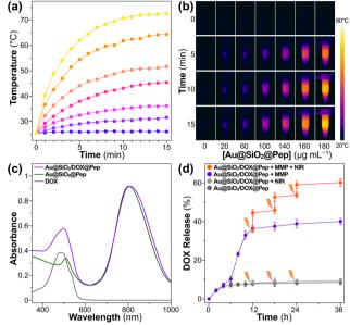
Fig. 2 (a and b) Temperature versus time curves and infrared thermographic images of Au@SiO2@Pep samples of different concentrations upon being exposed to NIR irradiation. (c) UV-Vis spectra of DOX, Au@SiO2/DOX, and Au@SiO2/DOX@Pep. (d) DOX release profiles of Au@SiO<sub>2</sub>/DOX@Pep at pH 6 upon being exposed to MMP and NIR stimuli.
