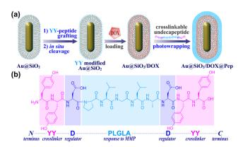
Scheme 1 (a) The fabrication of peptide-photowrapped Au@SiO<sub>2</sub>/DOX@ Pep nanocapsules, and (b) the design of crosslinkable undecapeptide.
