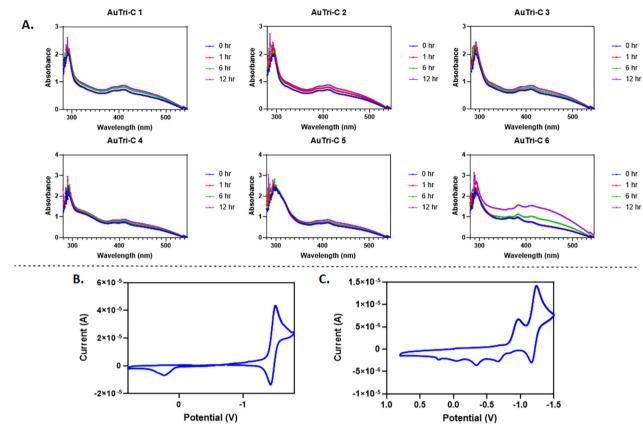
Fig. 2 (A) UV-vis absorption spectra of AuTri-C complexes in biologically relevant media, DMEM at 37 °C, final concentration of the complexes 50 µM. (B and C) Cyclic voltammogram recorded at a platinum electrode in DMSO solution of 5 mM AuTri-C-5 or AuTri-C-6 with 0.10 M N(Bu)<sub>4</sub>PF<sub>6</sub> supporting electrolyte at a scan rate of 0.1 V s<sup>-1</sup> using Ag/AgCl reference electrode at RT.
