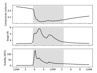
Fig. 5 Example aay with rainfall event. Shaded area indicates the type of signal changes that are associated with rainfall.
