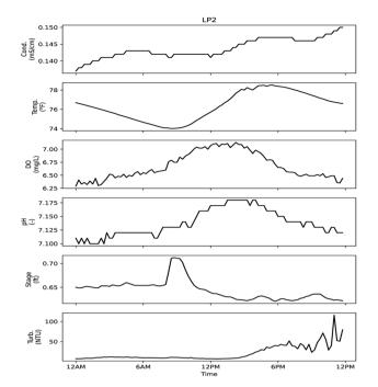
Fig. 10 Sensor signals during day of sample LP2. Low probability sampling event did not correspond to a triggered CANARY alarm. Sample collected at 9:09 AM.
