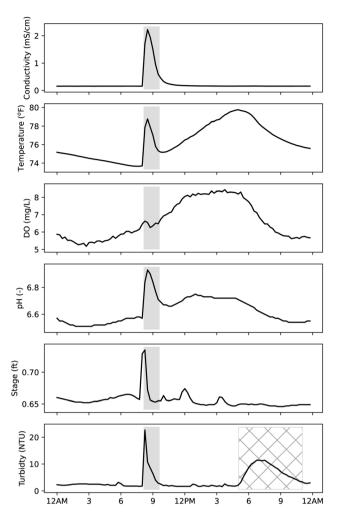
Fig. 6 Example day that triggered CANARY Alarm. Shaded area indicates the suspected illicit event and where CANARY alarms. Hatched area indicates approximate period with single sensor associated alarm.
