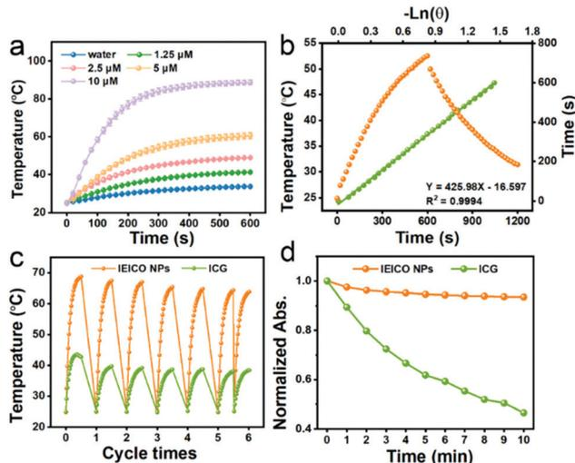
Fig. 2 (a) Time-dependent temperature variation of IEICO NP aqueous solutions with different concentrations under 808 nm laser irradiation (1 W cm<sup>-2</sup>). (b) Photothermal conversion efficiency of IEICO NPs. (c) The temperature changes of IEICO NPs (10 μM) and ICG (10 μM) in aqueous solutions under 808 nm laser for 6 cycles. (d) Time-dependent normalized absorbance of IEICO NPs and ICG.
