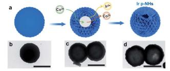
Fig. 1 (a) Schematic illustration of the structural evolution of Ir p-NHs, with corresponding TEM images of products collected at a reaction time of (b) 1 h, (c) 3 h and (d) 5 h. Scale bar, 1  $\mu$ m.
