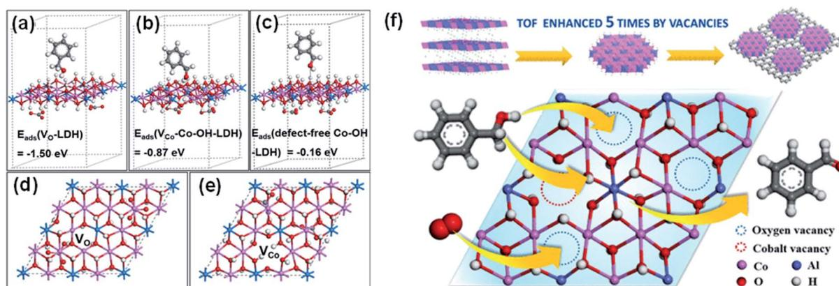
Fig. 22 DFT-calculated conformation of adsorption states and adsorption energies of a benzyl alcohol molecule on (a) an OV, (b) a  $V_{\text{Co}}\text{-Co-OH}$  site, and (c) defect-free Co-OH. Top views of the optimized structures of (d) an OV and (e) a Co vacancy. (f) Schematic diagram of Co-containing LDH for the aerobic oxidation of alcohols. Reproduced with permission. Adapted with permission from ref. 182 Copyright (2018) American Chemical Society.
