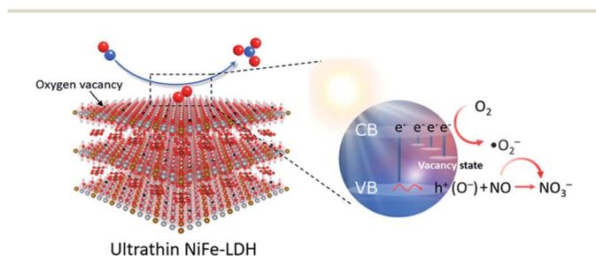
Fig. 6 Schematic illustration of activation of O<sub>2</sub> into O<sub>2</sub><sup>•-</sup> on NiFe-LDH with an OV for the selective photocatalytic oxidation of NO. Adapted with permission from ref. 140 Copyright (2022) American Chemical Society.
