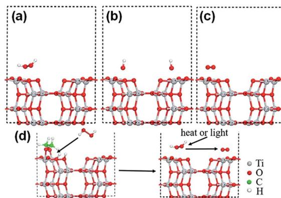
Fig. 5 Side view of (a)  $\text{H}_2\text{O}_2$  (b) initial configuration of two hydroxyl groups, and (c) superoxide radicals adsorbed on the  $\text{TiO}_2$  predicted by the GGA-TS method. (d) The decomposition mechanism of  $\text{H}_2\text{O}_2$  into superoxide radicals on  $\text{TiO}_2$  NSs. Adapted with permission from ref. 132 Copyright (2017) American Chemical Society.
