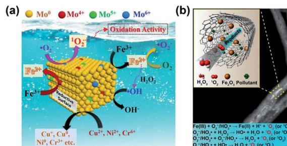
Fig. 9 (a) Schematic illustration of Mo catalytic oxidation of  $\text{O}_2^{\cdot-}$  to  $^1\text{O}_2$ . Adapted with permission from ref. 43 Copyright (2021) American Chemical Society. (b) Schematic illustration of the generation of  $^1\text{O}_2$  over  $\text{Fe}_2\text{O}_3@\text{FCNT-H}/\text{H}_2\text{O}_2$ . Adapted with permission from ref. 151 Copyright (2019) National Academy of Sciences.
