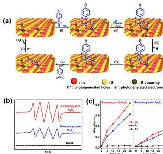
Fig. 17 (a) Proposed mechanism of the photooxidation of benzyl alcohol to benzaldehyde. (b) ESR spectra of SV-rich and SV-poor In<sub>2</sub>S<sub>3</sub> in the presence of DMPO. (c) The dramatically different oxidation rates of the indicator molecule 3,3',5,5'-tetramethylbenzidine in various gas environments (oxygen, air, and nitrogen) indicate that the ROS evolved from O<sub>2</sub>. Adapted with permission from ref. 147 Copyright (2019) American Chemical Society.
