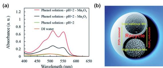
Fig. 4 (a) Detection of  $\text{H}_2\text{O}_2$  by activation of  $\text{O}_2$  over  $\text{Mn}_3\text{O}_4$  and  $\text{Mn}_2\text{O}_3$ , respectively. (b) Schematic illustration of the recycling strategy for  $\text{Mn}_3\text{O}_4$  and  $\text{Mn}_2\text{O}_3$  on  $\text{O}_2$  activation to generate  $\text{H}_2\text{O}_2$  that decomposes into  $\text{HO}^\cdot$ . Adapted from ref. 120 with permission from The Royal Society of Chemistry.
