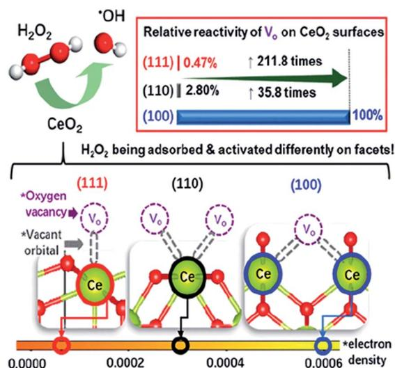
Fig. 3 Schematic illustration of the synergy effect of Ce and OVs on the  $CeO_2$  surface for the efficient activation of  $H_2O_2$  into  $HO^\bullet$ . Adapted with permission from ref. 118 Copyright (2020) American Chemical Society.
