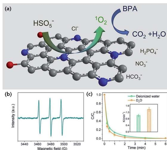
Fig. 18 (a) Schematic illustration of BPA degradation. (b) EPR spectrum of PMS activation. (c) Effect of D<sub>2</sub>O on BPA removal efficiency. Adapted with permission from ref. 275 Copyright (2019) Elsevier.
