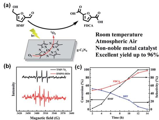
Fig. 20 (a) Possible mechanism of the photocatalytic oxidation of HMF with the CoPz/g-C<sub>3</sub>N<sub>4</sub> catalyst. (b) EPR signals of the DMPO-HO· adduct in water in the presence of bulk g-C<sub>3</sub>N<sub>4</sub> and the TMP-<sup>1</sup>O<sub>2</sub> adduct in water in the presence of CoPz/g-C<sub>3</sub>N<sub>4</sub> in the photocatalysis process. (c) Photocatalytic performance. Adapted with permission from ref. 287 Copyright (2017) American Chemical Society.
