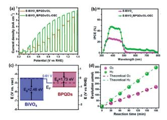
Fig. 11 (a) J-V curves of E-BiVO<sub>4</sub>/BPQDs/OL and E-BiVO<sub>4</sub>/BPQDs/ OL-OEC. (b) IPCE values of E-BiVO<sub>4</sub> and E-BiVO<sub>4</sub>/BPQDs/OL-OEC. (c) Band alignment diagram of E-BiVO<sub>4</sub> and BPQDs showing type II heterojunction. (d) HER and OER activities of the E-BiVO<sub>4</sub>/BPQDs/OL-OEC photoanode at 1.23 V vs. RHE. Reproduced with permission from ref. 133 © 2022 The Royal Society of Chemistry.
