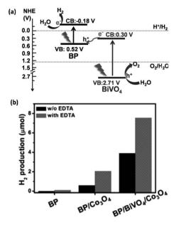
Fig. 10 (a) Schematic presentation of BP/BiVO<sub>4</sub> composite based Zscheme photocatalyst for visible and NIR radiation (>420 nm) induced overall water splitting. (b) H<sub>2</sub> evolved by different catalysts with and without Co<sub>3</sub>O<sub>4</sub> co-catalyst and EDTA sacrificial agent under >420 nm light irradiation. Reproduced with permission from ref. 118, © 2018 Wiley-VCH Verlag GmbH & Co. KGaA, Weinheim.
